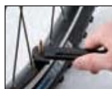
Offset wrench for the removal of rim nut
