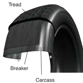
Cross section of a bias tire
